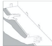
1. Begin installation from left to right. Install spacers at ends & where planks meet wall.
