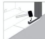
2. Use mallet and pull bar to tap in and lock short side of board.
